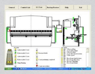
Simply edit the dimensions on the profile displayed before folding simulation is viewed. Identifying potential collisions.
