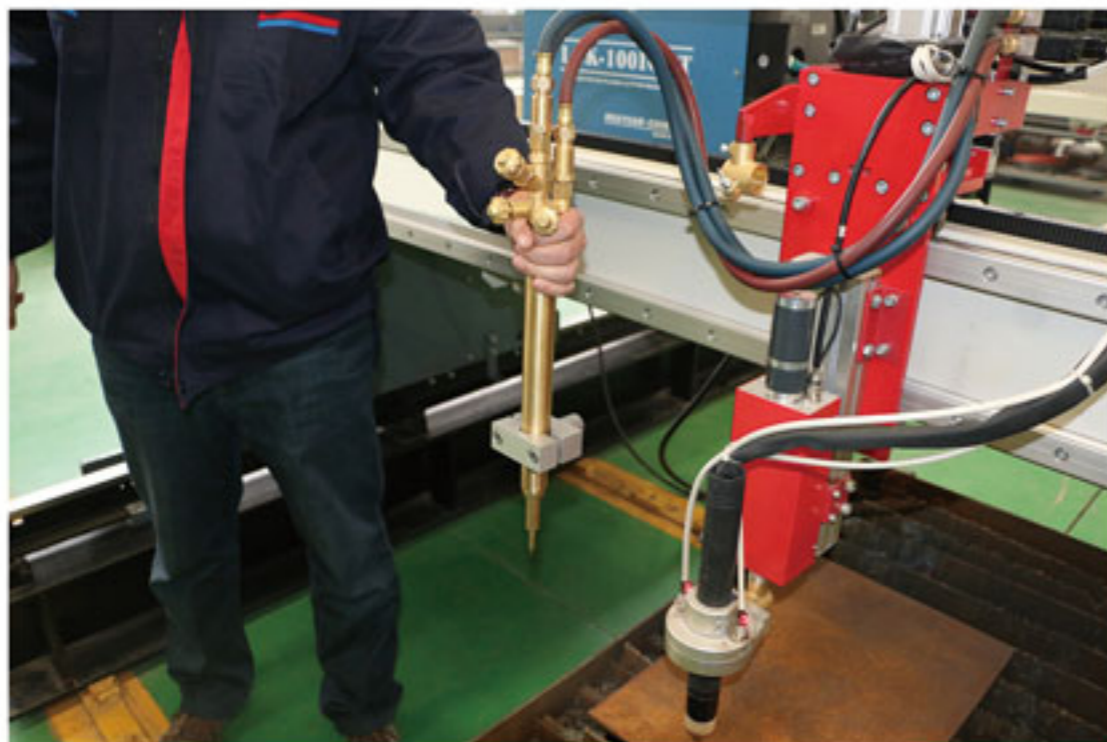
1. Easy change plasma and oxy-fuel configuration.
