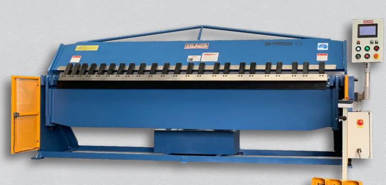
**STEELMASTER** Full hydraulic Panbrake folder models range from manual angle setting, 1 Axis NC angle controller, 2 Axis NC angle controller with ballscrew backgauge with roller table & full CNC 2 Axis machines. Produced exclusively for Asset by Australian Engineers.
