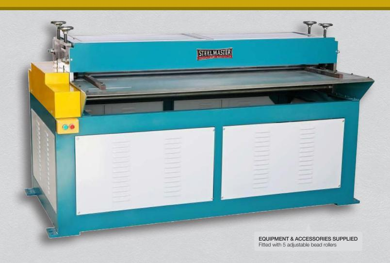
Our Rib Roller Roll former offers adjustable rib roller spacers allowing you to set your own rib width settings.
