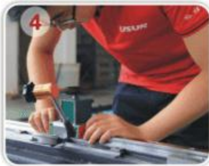
Straightness: using clock gauge to recheck guide line
