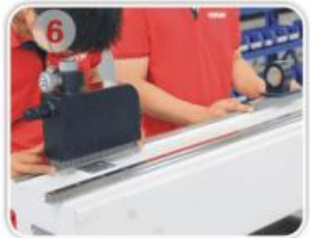
Straightness: using auto collimator to check beam
