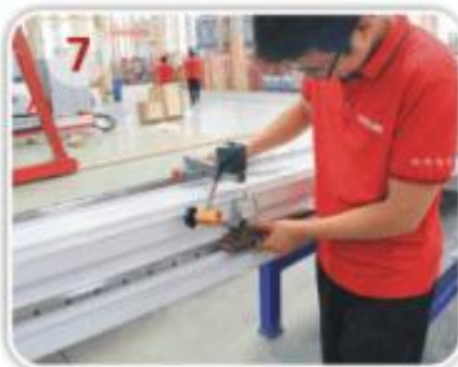
Straightness: using clock gauge to recheck guide line on beam
