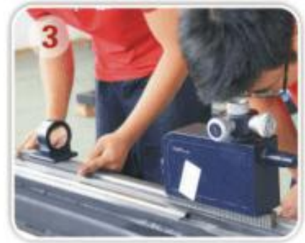
Straightness: using auto collimator to check frame
