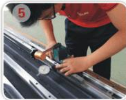
Flatness: using plug gauge to check the rack and gear
