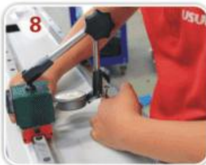
Flatness: using plug gauge to check the rack and gear on beam
