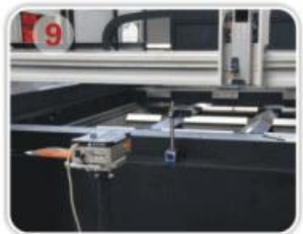
Precision: using interferometer to check X/Y stroke
